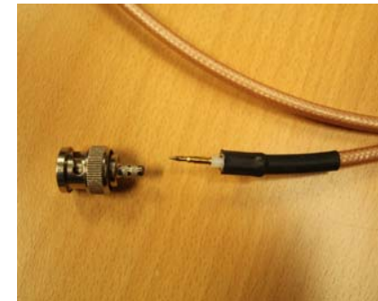
Typical cable system failure
