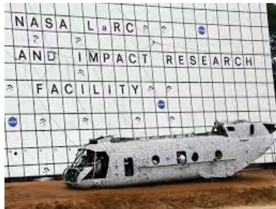
TRACT 1 Helicopter Crash Test at LandIR from 2013
