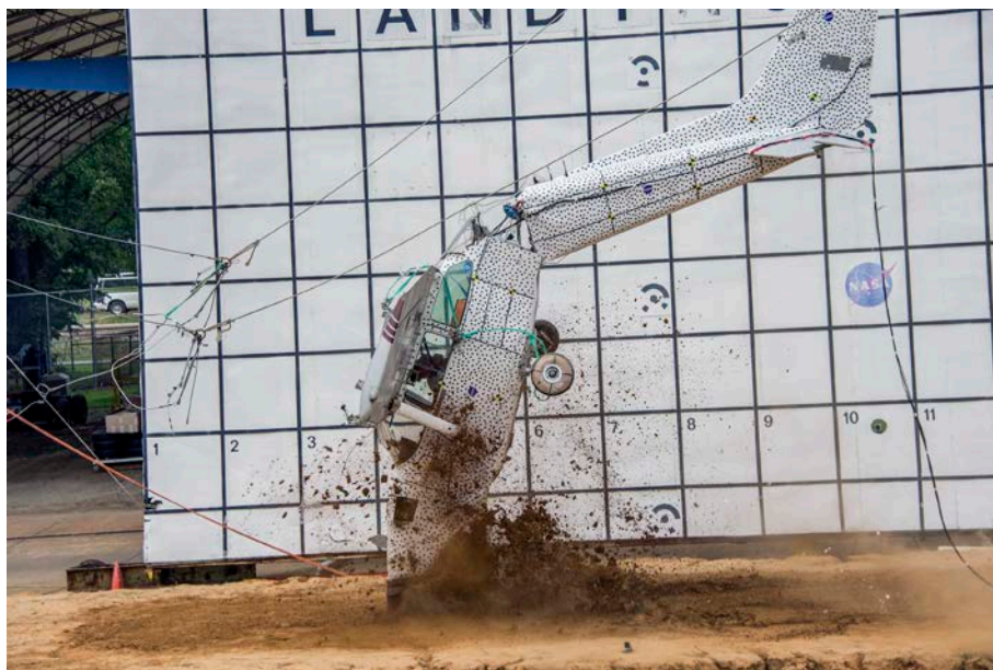
4 ELTs onboard: Cessna 172 Crash Test
