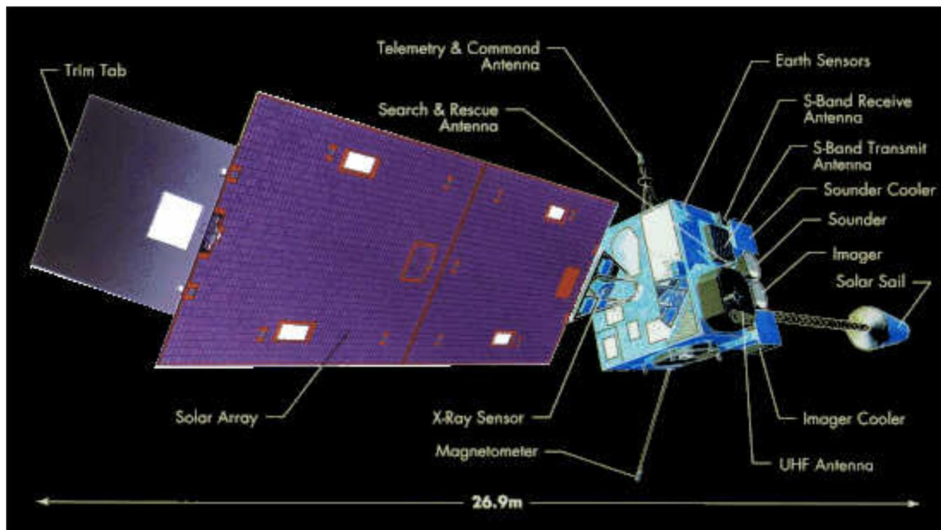
UHF Antenna receives 406-406.1 MHz signals and GOES Search and Rescue Repeater (SARR) retransmits band down via S&R antenna centered at 1544.5 MHz (LHCP)
